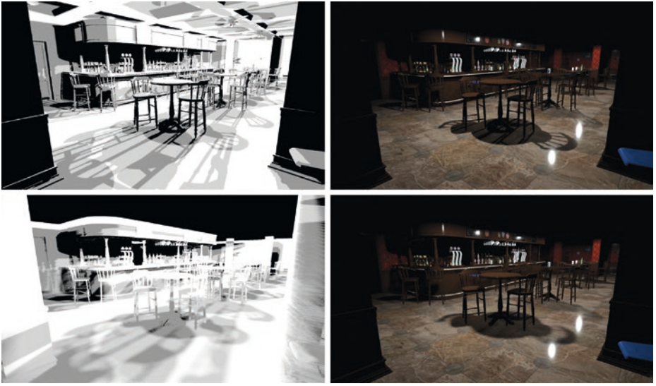
Figure 13-11. Hard shadows comparison. Visibility buffers (left) and rendered image (right) for the Pub scene with four lights, showing hard shadows rendered using our method (top) and shadow mapping (bottom).
