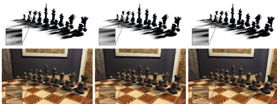
Figure 13-1. Left: soft shadows rendered using naive ray traced shadows with 4 samples per pixel running at 3.6 ms per frame. Center: soft shadows rendered using our adaptive method with 0 to 5 samples per pixel running at 2.7 ms per frame. Right: naive ray traced shadows using 256 samples per pixel running at 200 ms per frame. Times measured using a GeForce RTX 2080 Ti GPU. Top: visibility buffers. Bottom: final images.
