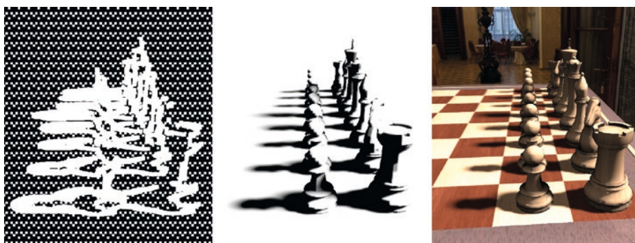
Figure 13-5. Left: image showing the pixels with nonzero sample counts. Note the sampling of the penumbra regions and the pattern enforced by the sampling matrix. Center: visibility buffer. Right: final image.
