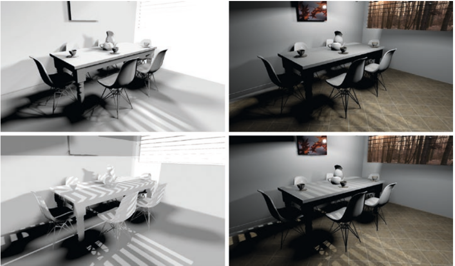
Figure 13-12. Soft shadows comparison. Visibility buffers (left) and rendered image (right) for the Breakfast scene with four lights, showing soft shadows rendered using our method (top) and shadow mapping (bottom).
